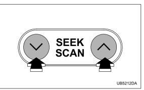
If you press the "  $\land$  " or "  $\lor$  " side of the SEEK/SCAN button for 1.5 second or longer, the radio will switch to scan mode. In this mode, the radio scans through the radio band until a station is found. The radio will stop at the station for five seconds while displaying the frequency, after which scanning will continue until the entire band has been scanned.
