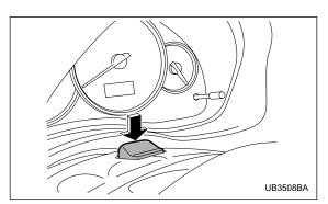
The parking light switch operates regardless of the ignition switch position.
