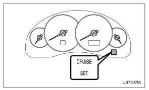
At this time, the "  $_{\rm SET}$  " indicator light is illuminated in the combination meter.
