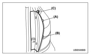
2. Wrap tape around a flat-head screwdriver, then insert the screwdriver into the gap A between the side cover and rear combination lamp and use it as a lever to undo the clip. Undo clips C and D in the same way, then remove the side cover.
