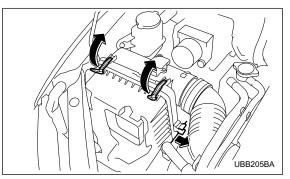
4. Unsnap the two clamps holding the air cleaner case cover.
