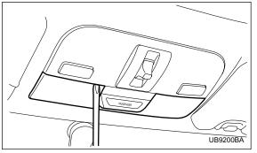
2. Remove the spotlight lens by prying the edge of the lens using flat-head screwdriver.
