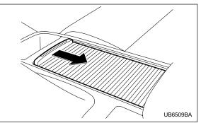
Slide the sliding lid (near the parking brake lever) toward the rear.
