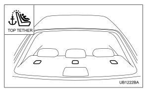
Three tether anchorages are installed on the rear shelf behind the rear seat head restraint. Open the cover flap to use each anchorage.
