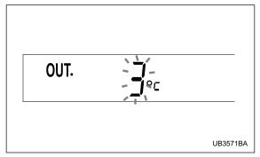
When the outside temperature drops to  $37^{\circ}F(3^{\circ}C)$  or lower, the temperature indication flashes to show that the road surface may be frozen.
