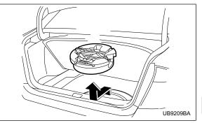
**Sedan:** To take out the jack and maintenance tools, open the floor cover and remove the bucket from the center of the spare tire. Then, take the jack out of the bucket.
