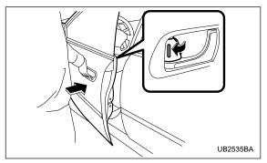
4. Before closing the doors, lock all doors with the inside door lock levers.
