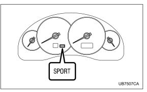
When selected, the SPORT mode indicator light on the instrument panel will turn on.
