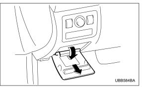
Open the lid that is located above the hood release knob and pull it toward you to remove it.
