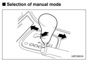
With the vehicle either moving or stationary, move the selector lever from the "D" position to the manual gate then move it to the "+" end or "-" end of the manual gate to select manual mode.
