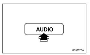
**To change tone control modes:** Each brief press of the "AUDIO" button changes control modes in the following sequence starting from volume control mode. (When the radio is first turned on, the control mode is in the volume control.)
