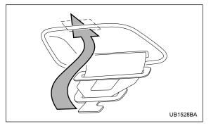
2. Allow the retractor to roll up the belt. You should hold the webbing end and guide it back into the retractor while it is rolling up. Neatly store the tongue plate in the recess in the retractor and then insert the connector (tongue) plate into the slot located at the front of the recess.
