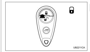
Press the " Press the " button to lock all doors and rear gate (Station wagon). An electronic chirp will sound once and the turn signal lights will flash once.
