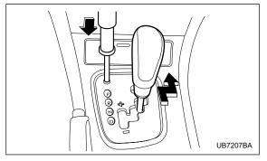
If you inadvertently have turned the ignition switch to the "OFF" position with the selector lever in the "N" position, proceed as follows. By referring to the "Shift lock release" section in this chapter, remove the shift lock release cover. Then, with the screwdriver inserted
