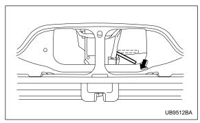
3. Unlock the rear gate by pressing the lever inside the trim downward.
