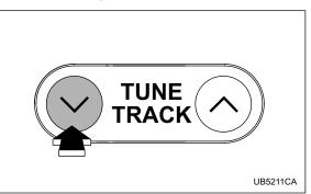
Press the "  $\,\,\bigtriangledown\,$  " side of the TUNE/TRACK button continuously for more than 0.5 second to fast-reverse the disc.
