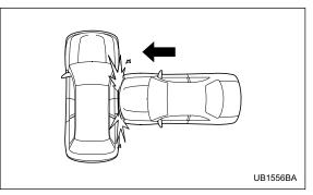
A severe side impact near the front seat activates the SRS side airbag and SRS curtain airbag.
