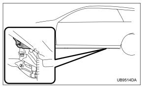
The rear tie-down hooks are located near each of the jack-up reinforcements.
