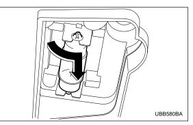
2. Turn the bulb until the flat surfaces at its ends are aligned vertically. Pull the bulb straight downward to remove it.
