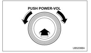
The dial is used for both power (ON/OFF) and volume control. The radio is turned ON and OFF by pushing the dial and the volume is controlled by turning the dial. The dial can also be used for tone and balance adjustment.
