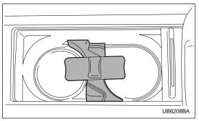
If you remove the divider plate from the dual cupholders, you can use the center console box as a storage space.
