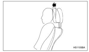
The front seats of your vehicle are equipped with active head restraints. They automatically tilt forward slightly in the event the vehicle is struck from the rear, decreasing the amount of rearward head movement and thus reducing the risk of whiplash. For maximum effectiveness the head restraint should be adjusted so that the center of the head restraint is closest to the top of the occupant's ears.
