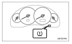
The tire pressure monitoring system provides the driver with a warning message indicated by sending a signal from a sensor that is installed in each wheel when tire pressure is severely low.
