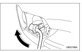
5. Tighten the towing hook securely by a wheel nut wrench.
