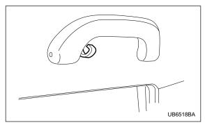
The coat hook is attached to each rear passenger's hand grip.
