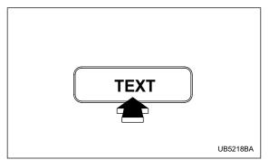
If you press the "TEXT" button for 0.5 second or longer during playback, the indication will change to the next one in the sequence shown below.
