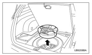
**Station wagon:** To take out the jack and maintenance tools, open the center lid and remove the bucket from the center of the spare tire. Then, take the jack out of the bucket.
