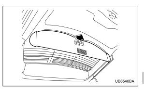
Rotate the rear gate board toward you until its top touches the rear gate panel.
