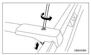
1. Loosen and remove the T-30 torx® head screw from the top of each crossbar end support. Loosen the lower clamps.
