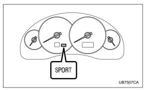
When selected, the SPORT mode indicator light on the instrument panel will turn on.
