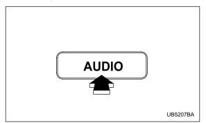
Each brief press of the "AUDIO" button changes control modes in the following sequence starting from volume control mode. (When the radio is first turned on, the control mode is in the volume control.)
