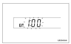
The journey time indication flashes each time a complete hour has elapsed. If the display is giving an indication other than the journey time, the display switches to the journey time, flashes for five seconds, and returns to its original indication each time a complete hour has elapsed.
