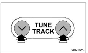
Press the "  $_{\bigwedge}$  " side of the TUNE/TRACK button to increase the tuning frequency and press the "  $_{\bigvee}$  " side of the button to decrease it.
