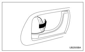
To unlock the door from the inside, rotate the lock lever forward.
