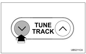
Briefly press the "  $\lor$  " side of the TUNE/TRACK button to skip to the beginning of the current track/file (track). Each time the button is pressed, the indicated track/file (track) number will decrease.
