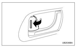
To lock the door from the inside, rotate the lock lever rearward.
