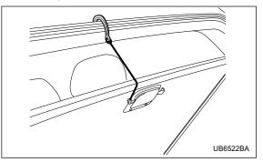
1. Open the lid and hang the hook provided on the under side of the lid on the rear edge of the roof to keep the lid open.
