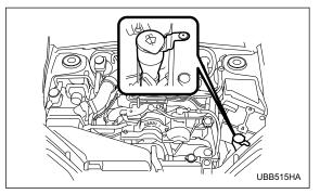
If you spray washer fluid on the windshield but the supply of washer fluid appears to diminish, check the level of washer fluid in the tank.
