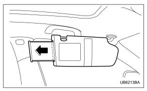
With the sun visor positioned over the side window, you can use the sun visor extension plate to prevent glare through the gap between the sun visor and center pillar. To use the extension plate, pull it toward the rear of the vehicle. When you have finished using it, stow it by pushing it toward the front of the vehicle.
