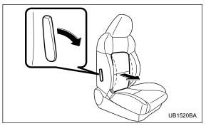
Pull the lever forward or backward. Pulling the lever forward will increase the amount of support for your lower back.
