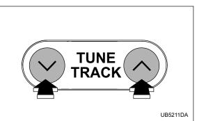
Push the "  $_{\wedge}$  " side of the TUNE/TRACK button to increase the tuning frequency and press the "  $_{\vee}$  " side of the button to decrease it.
