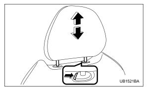
To raise the head restraint, pull it up. To lower it, push the head restraint down while pressing the release button on the top of the seatback.
