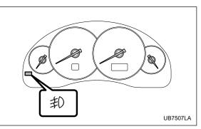
The indicator light located on the combination meter will illuminate when the fog lights are on.
