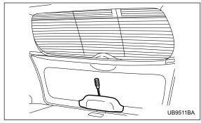
1. Remove the access cover at the bottom-center of the rear gate trim using flat-head screwdriver.
