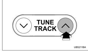
Press the "  $~\wedge~$  " side of the TUNE/TRACK button continuously for more than 0.5 second to fast-forward the disc.
