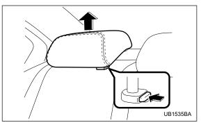
1. Remove the head restraint at the seating position where the child seat has been installed with the seatbelt or lower anchorages; lift up the head restraint while pressing the release button.
