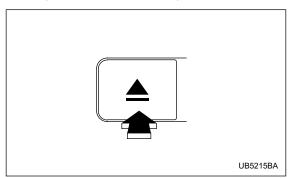
When a disc is being played back or when a disc is in the player, press the eject button "  $\blacktriangle$  ". The disc will be ejected.
