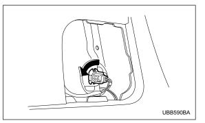
2. Turn the bulb socket counterclockwise and remove it.
