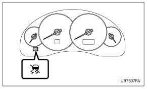
This single light has the function of indicating malfunctions in the Vehicle Dynamics Control system and the function of indicating that the Vehicle Dynamics Control system is not operating. It comes on in the event of a malfunction in the system and is illuminated whenever the system is not operating.
