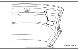
1. Use a flat-head screwdriver to remove the light cover from the top of the left hand rear gate trim.
