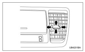
Move the tab up and down or right and left to adjust the flow direction.
