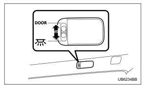
The cargo area light switch has three positions: **DOOR:** The light comes on only when the rear gate is opened.
