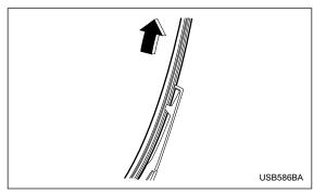
2. Pull the blade rubber assembly out of the plastic support.
