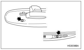
The mirror has a photosensor attached on both the front and back sides. If the glare from the headlights of
