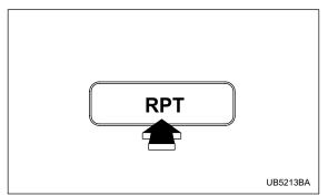
Use this to play a certain track repeatedly. During playback, press the "RPT" button. The "RPT" indicator will come on and the track will be played continuously. To cancel the repeat mode, press the button again. Then the "RPT" indicator goes out, and normal playback mode is restored.
