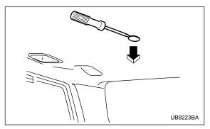
3. Remove the plug on the roof trim (located to the rear of the moonroof) by inserting the end of the fladbladed screwdriver between the roof and plug and prying it off.
