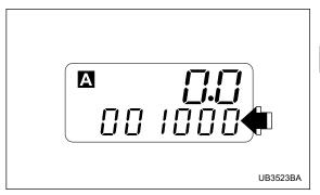
This meter displays the odometer when the ignition switch is in the "LOCK", "ACC" or "ON" position. The odometer shows the total distance that the vehicle has been driven.
