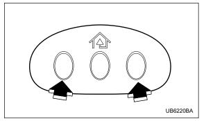
2. Press and hold the two outside buttons until the HomeLink® indicator light begins to flash (after 20 seconds). Release both buttons.
