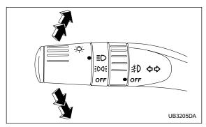
To activate the right turn signal, push the turn signal lever up. To activate the left turn signal, push the turn signal lever down. When the turn is finished, the lever will return automatically. If the lever does not return after cornering, return the lever to the neutral position by hand.
