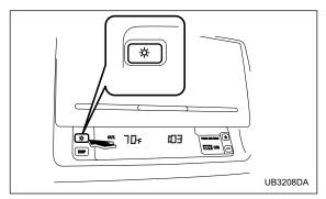
The brightness of clock display, audio, air conditioner, multi information display and instrument panel illumination dims when the light switch is in the " $\pm co \pm$ " or " $\equiv \bigcirc$ " positions.
