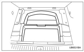
Hang the hook provided on the underside of the lid on the rear edge of the roof to keep the lid open.
