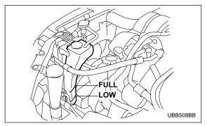
6. Pour the coolant and fill to the reservoir tank's "FULL" level mark.
