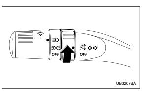
The front fog lights operate only when the light switch is in the "  $\exists D d \exists D$  " or "  $\exists D$  " position.
