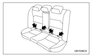
The lower anchorages (bars) are used for installing a child restraint system only on the rear seat window-side seating positions. For each window-side seating position, two lower anchorages are provided. Each lower anchorage is located where the seat cushion meets the seatback.
