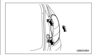
3. Remove the upper and lower screws. Then, slide the rear combination lamp assembly to the rear and remove it from the vehicle.
