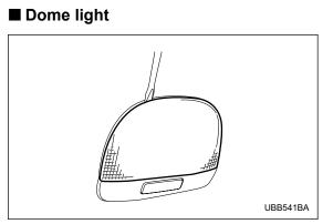
1. Remove the lens by prying the edge of the lens with a flat-head screwdriver.
