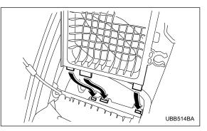
7. To install the air cleaner case cover, insert the three projections on the air cleaner case cover into the slits on the air cleaner case and then snap the two clamps on the air cleaner case cover.
