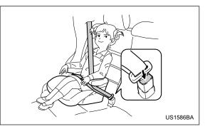
4. To remove the booster seat, press the release button on the seatbelt buckle and allow the belt to retract.
