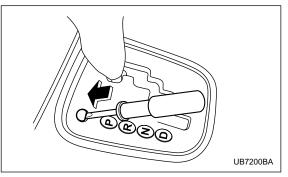
3. Remove the cover by prying on the edge with a flathead screwdriver.
