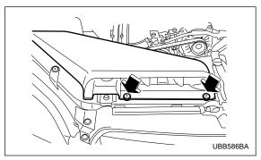
1. Use a screwdriver to undo the clips on the air intake duct, then remove the air intake duct.
