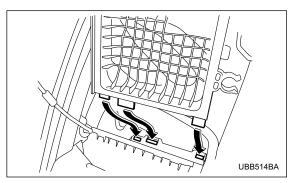
7. To install the air cleaner case cover, insert the three projections on the air cleaner case cover into the slits on the air cleaner case and then snap the two clamps on the air cleaner case cover.
