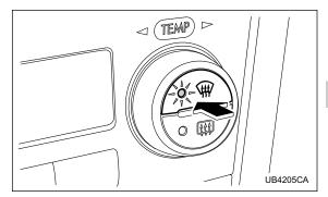
To defrost or dehumidify the windshield and front door windows, push the defroster button " $\langle H H \rangle$ ". When the " $\langle H H \rangle$ " button is pushed, regardless whether the air conditioner is operating or not, outside air is drawn into the passenger compartment, the air conditioner compressor turns on, air flow is directed towards the windshield and front door windows, and the indicator light on the button comes on.
