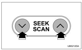
The scan mode lets you listen to the first 10 seconds of each track/file (track) in succession. Press the " $\land$ " side of the SEEK/SCAN button for 1.5 second or longer to start scanning upward beginning with the track/ file (track) following the currently selected one. Press
