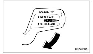
Push the control lever downward in the "SET/COAST" direction and hold it until the vehicle reaches the desired speed. Then, release the control lever. The vehicle speed at that moment will be memorized and treated as the new set speed.
