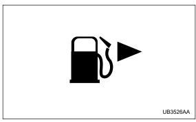
• You will see the " IN> " sign in the combination meter. This indicates that the fuel filler door (lid) is located on the right side of the vehicle.
