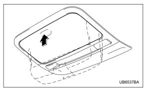
To open the console, push on the lid lightly and it will automatically open.
