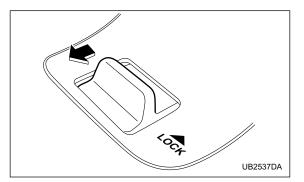
6. When you have finished entering the number, pull the lock knob to the "UNLOCK" side within five seconds.
