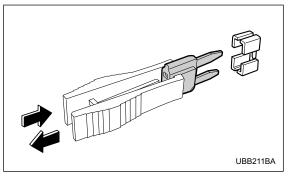
4. Pull out the fuse with the fuse puller.
