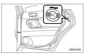
Each rear door has a child safety lock that prevents the doors from being opened even if the inside door handle is pulled. When the child safety lock lever is in the lock position, the door cannot be opened from inside regardless of the position of the inner door handle lock lever. The door can only be opened from the outside.
