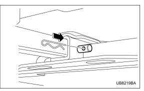
3. Insert the safety pin into the hitch pin securely.
