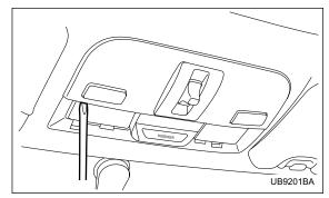
3. Remove the two screws that retain the moonroof switch body. Then, remove the moonroof switch.
