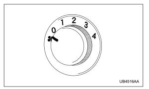
The fan operates only when the ignition switch is turned to the "ON" position. The fan speed control dial is used to select four fan speeds.
