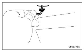
4. Insert the wrench in the end of the motor shaft. To close the moonroof, turn the wrench clockwise.
