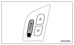
This button is used to select the desired audio mode. Each time it is pressed, the mode changes to the next one in the following sequence:
