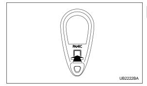
A "PANIC" button is located on the back of the transmitter.
