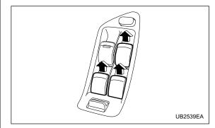
To close the window, pull the switch up and hold it until it reaches the desired position.
