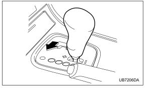
SPORT mode is used when power is needed for rapid acceleration or for uphill driving. To select this mode, move the selector lever from the "D" position to the manual gate.
