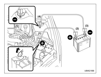
1)Connect one jumper cable to the positive (+) terminal on the discharged battery.
