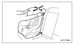
5. Before seating a child in the child restraint system, try to move seat back and forth and left and right to verify that it is held securely in position.
