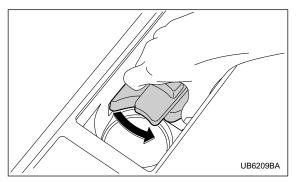
Grasp the dual cupholders' divider plate at the base. Turn it counterclockwise to remove it.
