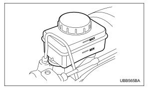
Check the fluid level on the outside of the reservoir. If the level is below "MIN", add the recommended brake fluid to "MAX".
