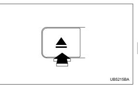
1. If you continue to press the "▲" button, the player will produce beep sound and will enter the all disc ejection mode. At this time, the disc number indicator and "ALL EJECT" indicator will flash.
