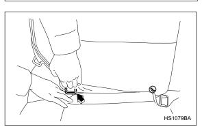
1. **Sedan:** Make the clearance between the seat cushion and seatback a little wider to locate the two anchorages (bars) for the position where you want to install the child restraint system.
