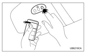
4. Using both hands, simultaneously push the handheld transmitter button and the desired HomeLink® button. DO NOT release the buttons until step 5 has been completed.
