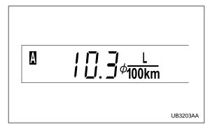
This indication shows the average rate of fuel consumption since the trip meter was last reset.
