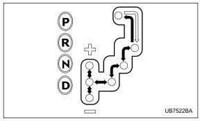
: Shift possible with brake pedal depressed
