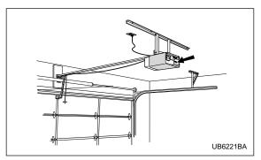
1. Locate the training button on the garage door opener motor head unit. The exact location and color of the button may vary by brand of garage door opener. If it is difficult to locate the training button, refer to your garage door opener's instruction manual.
