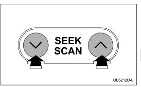
If you press the "  $\wedge$  " or "  $\vee$  " side of the SEEK/SCAN button for 1.5 second or longer, the radio will switch to scan mode. In this mode, the radio scans through the radio band until a station is found. The radio will stop at the station for five seconds while displaying the frequency, after which scanning will continue until the entire band has been scanned from the low end to the high end.
