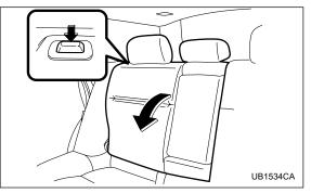
Unlock the seatback by pushing the release button and then fold the seatback down.
