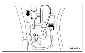
4. Insert the screwdriver into the hole.
