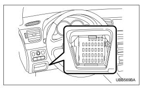
The fuses are designed to melt during an overload to prevent damage to the wiring harness and electrical equipment. The fuses are located in two fuse boxes. One is located under the instrument panel behind the fuse box cover on the driver's seat side.
