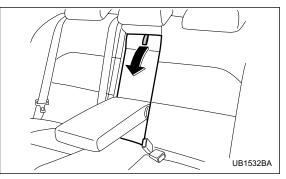
Folding down the armrest and opening the seatback panel affords a loading space for long objects. To open the seatback panel, pull the panel down while pressing the release tab down.
