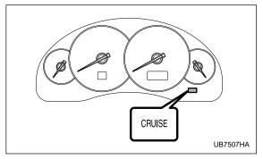
The cruise control indicator light comes on when the ignition switch is turned to the "ON" position and goes out after about three seconds.
