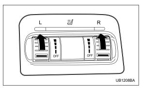
The seat heater operates when the ignition switch is either in the "ACC" or "ON" position.
