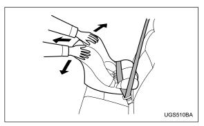
6. Push and pull the child restraint system forward and from side to side to check if it is firmly secured. Sometimes a child restraint can be more firmly secured by pushing it down into the seat cushion and then tightening the seatbelt.
