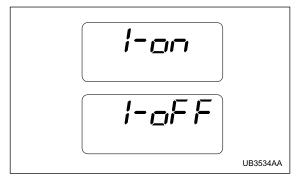
Briefly press the trip knob again. You can now establish the activated/deactivated setting for sequential illumination of the combination meter when the ignition switch is turned to the "ON" position. To change the current setting, press the trip knob for at least two seconds.
