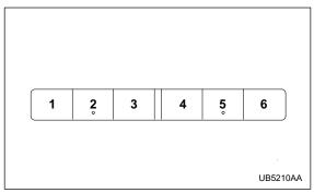
1. Use the disc select button to select the disc to be ejected.
