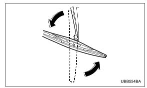
2. Turn the wiper blade assembly counterclockwise.
