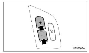
Press the "+" button to increase the volume. Press the "-" button to reduce the volume.
