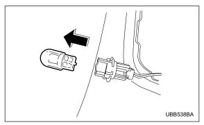
3. Pull the bulb out of the bulb socket and replace it with a new one.
