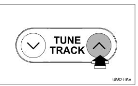
Press the "  $_{\bigwedge}$  " side of the TUNE/TRACK button continuously for more than 0.5 second to fast-forward the disc/folder.
