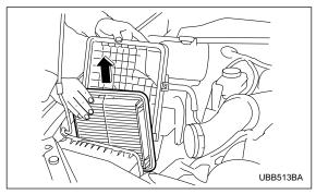
5. Open the air cleaner case cover and remove the air cleaner element.
