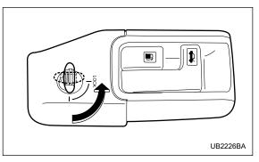
When you entrust your vehicle key to another person, you can lock the trunk lid release lever to prevent luggage in the trunk from being stolen. To lock the trunk lid release lever, insert the master key or sub key into the key cylinder at the rear of the release lever and turn it counterclockwise. To unlock the trunk lid release lever, turn the key clockwise.
