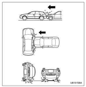
The driver's and front passenger's SRS frontal airbags are designed basically not to deploy if the vehicle is – CONTINUED –
