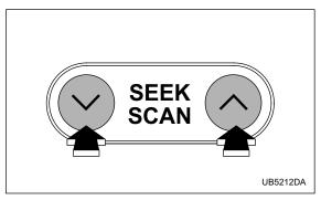
If you press the " $_{\wedge}$ " or " $_{\vee}$ " side of the SEEK/SCAN button and release it within 1.5 second, the radio will automatically search for a receivable station and stop at the first one it finds. This function may not be available, however, when radio signals are weak. In such a situation, perform manual tuning to select the desired station.
