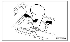
With the vehicle either moving or stationary, move the selector lever from the "D" position to the manual gate then move it to the "+" end or "–" end of the manual gate to select manual mode.
