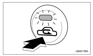
ON position (Recirculation): Interior air is recirculated inside the vehicle.
