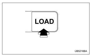
1. If you continue to press the "LOAD" button for more than 1.5 seconds, the player will produce beep sound and will enter the full disc loading mode.
