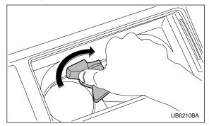
Insert the protrusion on the back of the divider plate into the hole in the center of the console box. Grasp the divider plate at the base, and turn it clockwise to fit it.
