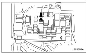
The fuse puller is stored in the main fuse box in the engine compartment.
