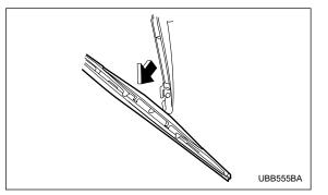
3. Pull the wiper blade assembly toward you to remove it from the wiper arm.
