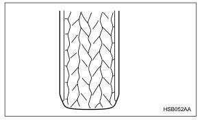
Roadholding is good, and steering is responsive. Rolling resistance is low, so fuel consumption is also lower. • Abnormally low tire pressure (tread worn at shoulders)
