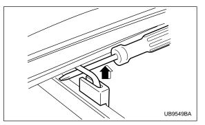
2)Use a screwdriver or similar implement to separate the slider and rod. Slide the sun shade toward the front of the vehicle.
