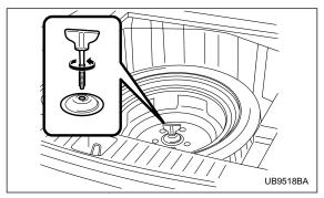
6. Turn the attaching bolt counterclockwise, then take the spare tire out.
