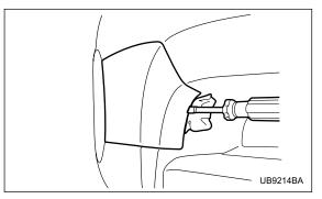
Wrap a flat-head screwdriver in a vinyl tape or cloth, insert it into the gap between the cover and the front bumper, and use it to lever the cover open.
