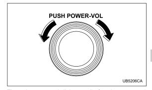
The volume control dial normally functions as a volume control. This dial becomes a control for Bass, Midrange, Treble, Fader or Balance when you select the appropriate tone and balance control mode. Choose desired volume level for each mode by turning the volume control dial. The control function returns to volume control mode after about 5 seconds.
