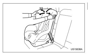
6. Before having a child sit in the child restraint system, move it back and forth and right and left to check if it is firmly secured. Sometimes a child restraint can be more firmly secured by pushing it down into the seat cushion and then tightening the seatbelt.
