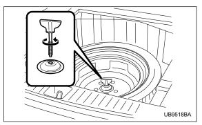
6. Turn the attaching bolt counterclockwise, then take spare tire out.
