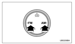
Push the "FM" or "AM" button when the radio is off to turn on the radio.
