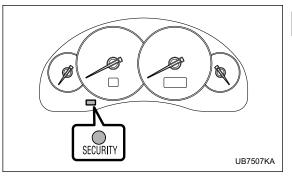
The security indicator light deters potential thieves by indicating that the vehicle is equipped with an immobilizer system. It begins flashing about 60 seconds after the ignition switch is turned from the "ON" position to the "ACC" or "LOCK" position or immediately after the key is pulled out.
