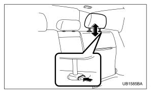
1. Remove the head restraint at the seating position where the child restraint system has been installed with the seatbelt or lower anchorages; lift up the head restraint while pressing the release button. Store the head restraint in the cargo area. Avoid placing the head restraint in the passenger compartment to prevent it from being thrown around in the passenger compartment in a sudden stop or a sharp turn.
