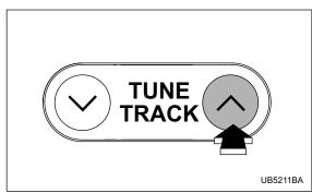
Briefly press the "  $_{\wedge}$  " side of the TUNE/TRACK button to skip to the beginning of the next track. Each time this side of the button is pressed, the indicated track number will increase.
