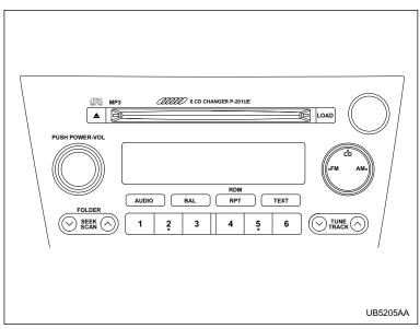
The audio set will operate only when the ignition switch is in the "ACC" or "ON" positions.
