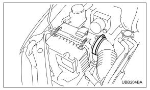
3. Use a screwdriver to remove the duct that is connected to the air cleaner case cover.
