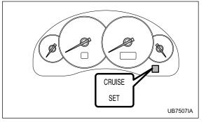
The cruise control set indicator light comes on when the ignition switch is turned to the "ON" position and goes out after about three seconds. The light comes on when vehicle speed has been set.
