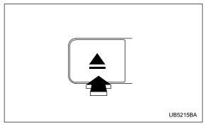
2. Briefly press the "▲" button. The selected disc will be ejected. The disc number indicator will flash at this time. When you remove the ejected disc, the disc number indicator will go off.
