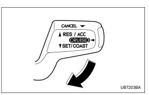
3. Push the control lever downward in the "SET/ COAST" direction and release it. Then release the accelerator pedal.
