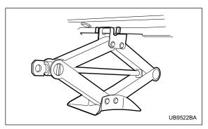
Turn the jackscrew by hand until the jack head engages firmly into the jack-up point.
