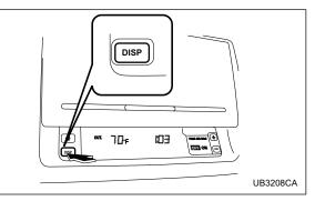
The clock will also show the time if you press the "DISP" button while the ignition switch is in the "OFF" position. It is possible to adjust the time setting while the time is being shown. If you do not press the "+" button or "-" button for 10 seconds while the time is being shown, the time indication will go off.
