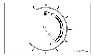
The rim of the fuel gauge flashes five time when the amount of remaining fuel reaches 2.6 US gal (10 liters, 2.2 lmp gal).
