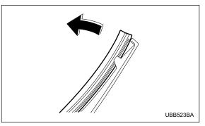
1. Pull out the end of the blade rubber assembly to unlock it from the plastic support.
