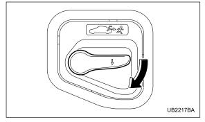
To open the trunk lid from inside the trunk, press the yellow handle downward as indicated by the arrow on the handle. This operation unlocks the trunk lid. Then, push up the lid.
