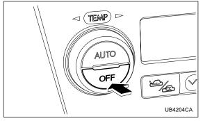
The Automatic Climate Control system turns off (the air conditioner compressor and fan turn off) when the "OFF" button is pressed.
