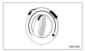
This dial regulates the temperature of air flow from the air outlets over a range from the blue side (cool) to red side (warm).
