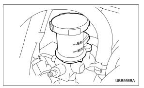
Check the fluid level on the outside of the reservoir. If the level is below "MIN" level mark, add the recommended clutch fluid to "MAX" level mark. Use only clutch fluid from a sealed container.
