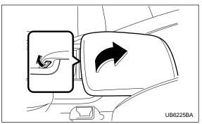
Pull up the lock release knob at the bottom of the front edge of the lid.
