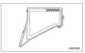
The spare fuses are stored in the main fuse box cover in the engine compartment.
