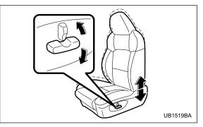
To adjust the seat height, pull up or push down the rear end of the control switch.
