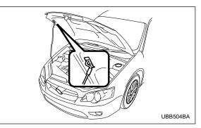
4. Lift up the hood, release the hood prop from its retainer and put the end of the hood prop into the slot in the hood.
