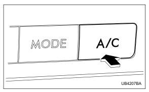
If the windshield starts to fog when the climate control system is operated in the AUTO mode, push the air conditioner button "A/C" to defog and dehumidify. When this button is pushed, the air conditioner compressor turns on and the indicator light "A/C" on the display comes on. After eliminating the fogging from the windshield, set the system back to the AUTO mode by pushing the "AUTO" button.
