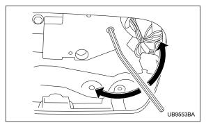
4. Insert the wrench in the end of the motor shaft. To lower the moonroof, turn the wrench clockwise. To close the moonroof, turn the wrench counterclockwise.
