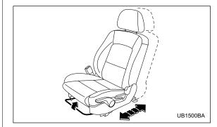
Pull the lever upward and slide the seat to the desired position. Then release the lever and move the seat back and forth to make sure that it is securely locked into place. Reclining the seatback
