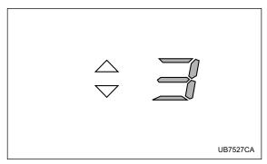
When the manual mode is selected, the gear position indicator (which shows the current gear selection) and the upshift/downshift indicator light up. (Refer to the "Automatic transmission -4 speed" or "Automatic transmission -5 speed" section in chapter 7.)
