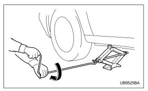
9. Insert the jack handle into the jackscrew, and turn the handle until the tire clears the ground. Do not raise the vehicle higher than necessary.
