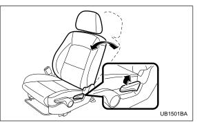
Pull the reclining lever up and adjust the seatback to the desired position. Then release the lever and make sure the seat is securely locked into place.
