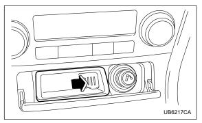
To remove the ashtray for cleaning, hold the right and left sides of the ashtray and pull it out.
