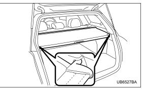
To extend the cover, pull the end of the cover out of the housing, then insert its hooks into the catches as shown. To rewind it, unhook it from the catches and it will rewind automatically. You should hold on to the cover and guide it back into the cover housing while it
