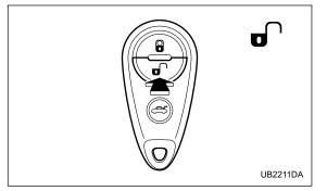
Press the "  $\bullet$  " button to unlock the driver's door. An electronic chirp will sound twice and the turn signal lights will flash twice. To unlock all doors and rear gate (Station wagon), briefly press the "  $\bullet$  " button a second time within 5 seconds.
