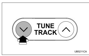
Press the "  $\,\,\bigtriangledown\,$  " side of the TUNE/TRACK button continuously for more than 0.5 second to fast-reverse the disc/folder.
