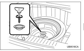
15. Store the flat tire in the spare tire compartment. Put the spacer and tighten the attaching bolt firmly. Also store the jack and jack handle in their storage lo-
