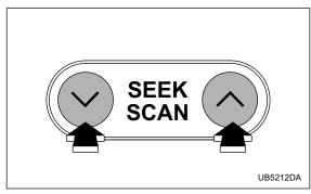
If you press the "  $_{\bigwedge}$  " or "  $_{\bigvee}$  " side of the SEEK/SCAN button and release it within 1.5 second, the radio will automatically search for a receivable station and stop at the first one it finds. This function may not be available, however, when radio signals are weak. In such a situation, perform manual tuning to select the desired station.
