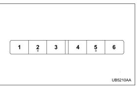
1. Use the disc select button to select the disc to be ejected.
