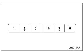
Press a desired one of the "Disc select" buttons the disc number indicator of which steadily lights up. The player will then start playback of the selected CD, beginning with the first track.
