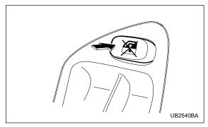
To lock the passengers' windows, push the lock switch. When the lock switch is in the "LOCK" position, the passengers' windows cannot be opened or closed.
