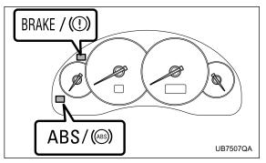
If a malfunction occurs in the EBD system, the system stops working and the brake system warning light and ABS warning light come on simultaneously.
