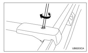
6. Adjust the alignment of the crossbar on the roof rails, and if available, use a T-30 torx® bit and torque wrench and tighten the T-30 torx® head screws to 30 to 35 lbf-in (3.4 to 4.0 N·m, 0.35 to 0.41 kgf·m) of torque (or tighten securely with the torx® wrench provided).
