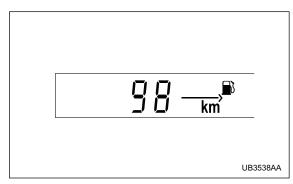
The driving range indicates the distance that can be driven taking into account the amount of fuel remaining in the tank and the average rate of fuel consumption.
