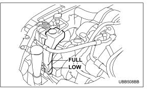
Check the coolant level at each fuel stop.
