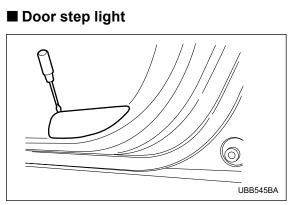
1. Remove the lens by prying the edge of the lens with a flat-head screwdriver.
