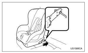
2. While following the instructions supplied by the child restraint system manufacturer, connect the lower hooks onto the lower anchorages located at " S" marks on the bottom of the rear seatback. When the hooks are connected, make sure the adjacent seatbelts are not caught.
