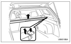
Hold down the button on the right hand rear quarter panel and lift up the right hand cover housing.
