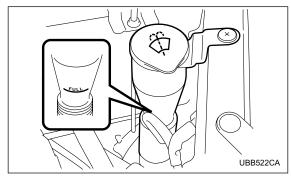
Remove the washer tank filler cap, then check the fluid level indicated by the level gauge (attached to the inside of the cap). If the level is near the "Low" mark, add fluid until it reaches the "Hi" level on the level gauge or the "Full" mark on the tank.
