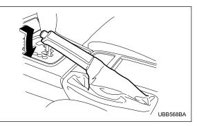
Check the parking brake stroke according to the maintenance schedule in the "Warranty and Maintenance Booklet". When the parking brake is properly adjusted, braking power is fully applied by pulling the lever up five to six notches gently but firmly (about 44 lbs, 196 N, 20 kg). If the parking brake lever stroke is not within the specified range, have the brake system checked and adjusted at your SUBARU dealer.
