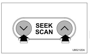
The scan mode lets you listen to the first 10 seconds of each track on the disc in succession. Press the " $\lor$ " side of the SEEK/SCAN button to start scanning through all tracks upward beginning with the track following the currently selected one. Press the " $\land$ " side of the button to start scanning through all tracks downward beginning with the track preceding the currently selected one. After all tracks on the disc have been scanned, normal playback mode is restored.
