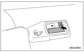
Pull the trunk lid release lever upward.
