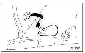
A retaining pin is located on the driver's side of the vehicle next to the fuel filler door release. Fit the grommet in the carpet onto the pin to prevent the carpet from moving.
