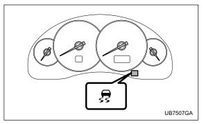
The indicator light turns on when the ignition key is turned to the ON position; it turns off approximately two seconds later. This indicator light flashes during activation of the skid suppression function and is illuminated steadily during activation of the traction control function.
