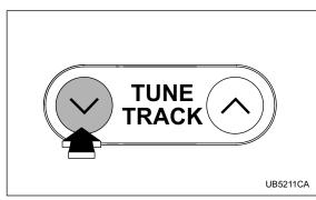
Briefly press the "  $\lor$  " side of the TUNE/TRACK button to skip to the beginning of the current track. Each time the button is pressed, the indicated track number will decrease.
