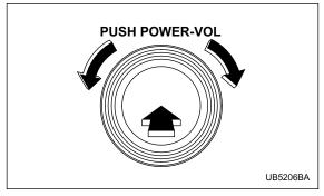
The dial is used for both power (ON/OFF) and volume control. The radio is turned ON and OFF by pushing the dial and the volume is controlled by turning the dial.
