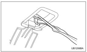
3. Fasten the top tether hook of the child restraint system to the appropriate upper anchorage.
