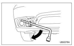
6. Tighten the towing hook securely by a wheel nut wrench.
