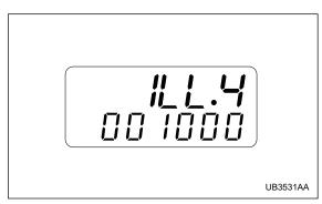
When the control dial is turned upward or downward, the instrument panel's illumination brightness is indicated by the trip meter. The brightness is shown in six steps from "*ILL. I*" (dimmest) to "*ILL.E*" (brightest).
