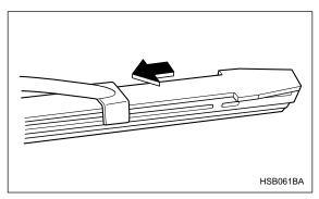
3. Align the claws of the metal support with the grooves in the rubber and slide the blade rubber assembly into the metal support until it locks.
