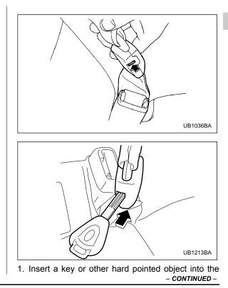
slot in the connector (buckle) on the right hand side and push it in, and the connector (tongue) plate will disconnect from the buckle.
