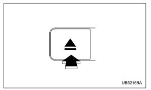
2. Briefly press the "  $\triangle$  " button. The selected disc will be ejected. The disc number indicator will flash at this time. When you remove the ejected disc, the disc number indicator will go off.
