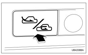
Select air flow by pushing the air inlet selection button " 2 2 .
