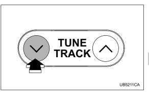
Briefly press the "  $\lor$  " side of the TUNE/TRACK button to skip to the beginning of the current track. Each time this side of the button is pressed, the indicated track number will decrease.
