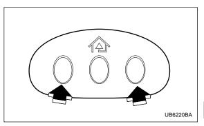
2. Press and hold the two outside HomeLink® buttons until the indicator light begins to flash (after 20 seconds). Release both buttons.
