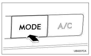
Select the desired air flow mode by pushing the air flow mode selection button. The selected air flow mode is shown by the display.
