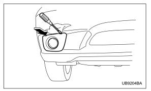
2. Wrap a flat-head screwdriver with cloth or vinyl. Then, insert the screwdriver into the gap between the fog light cover and the bumper, and pry out the cover.
