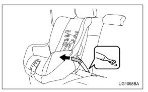
3. [If your child restraint system is of a flexible attachment type (which uses tether belts to connect the child restraint system properly to the lower anchorages)] While pushing the child restraint into the seat cushion, pull both left and right lower tether belts up to secure the child restraint system firmly by taking up the slack in the belt.
