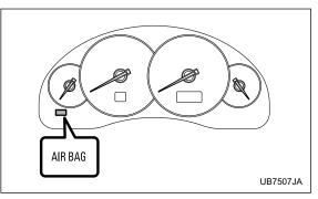
A diagnostic system continually monitors the readiness of the SRS airbag system (including front seatbelt pretensioners) while the vehicle is being driven. The SRS airbag system warning light "AIRBAG" will show normal system operation by lighting for about 6 seconds when the ignition key is turned to the "ON"
