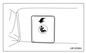
**Station wagon:** Remove the two covers from the selected side of the rear seatback to expose the anchorages (bars) to be used for installation of the child restraint system.
