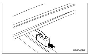
1)Push the slider at the rear of the rear moonroof frame toward the rear of the vehicle.
