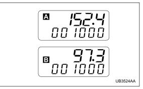
This meter displays the two trip meters when the ignition switch is in the "LOCK", "ACC" or "ON" position. The trip meter shows the distance that the vehicle has been driven since you last set it to zero.
