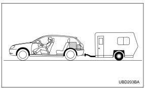
Vehicle capacity weight of the vehicle is 800 lbs (363 kg), which is indicated on the vehicle placard with the statement "The combined weight of occupants and cargo should never exceed 363 kg or 800 lbs".
