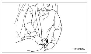
5. Insert the center seatbelt tongue plate in the center seatbelt buckle marked "CENTER" on the left hand side until it clicks.
