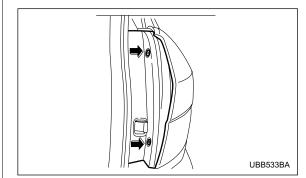
1. Using a Phillips screwdriver, remove the upper and lower screws.
