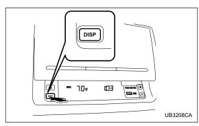
With the ignition switch in the "ON" position, each successive push of the "DISP" button toggles the display in the following sequence:
