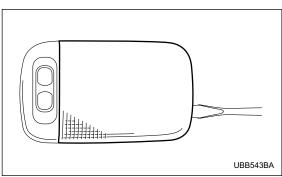
1. Remove the cargo area light assembly by prying the edge of the light with a flat-head screwdriver.
