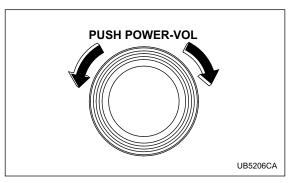
The volume control dial normally functions as a volume control. This dial becomes a control for Bass, Midrange, Treble, Fader or Balance when you select the appropriate tone and balance control mode. Choose desired volume level for each mode by turning the volume control dial. The control function returns to volume control mode after about 5 seconds.
