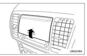
To open the center panel compartment, pull up the edge of the bottom of the panel lid.
