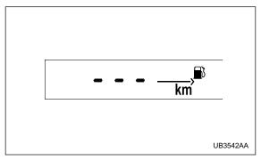
If the driving range is shown as "\_\_\_\_\_", there is only a tiny amount of fuel left in the tank. You must refuel the vehicle immediately.
