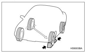
4. Put wheel blocks at the front and rear of the tire diagonally opposite the flat tire.
