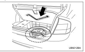
**Sedan:** Open the floor cover and remove the jack handle from the back of the floor cover.
