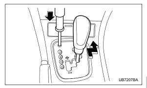
If you inadvertently have turned the ignition switch to the "OFF" position with the selector lever in the "N" position, proceed as follows. By referring to the "Shift lock release" section in this chapter, remove the shift lock release cover. Then, with the screwdriver inserted into the hole, move the selector lever to the "P" position. If the selector lever reverse inhibiting function fails, have the vehicle inspected by the nearest SUB-ARU dealer.
