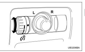
When the lighting switch is in the " $\exists OO\Xi$ " or " $\equiv O$ " position, you can adjust brightness of the instrument panel illumination for better visibility.
