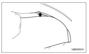
Fit the top of the rear gate board into the groove in the rear gate panel.
