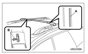
3. The crossbar with the 100 LBS Load Label attached onto it is the front crossbar. An arrow is marked on the back of the front crossbar for correct installation. Install the front crossbar so that the arrow faces the front of the vehicle.
