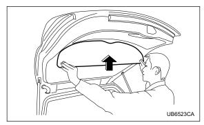
Insert (tipped at an angle) the hooks on the rear gate board into the holes in the rear gate panel.
