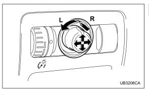
The remote control mirrors operate only when the ignition switch is in the "ON" or "ACC" position.
