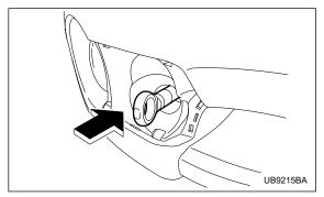
4. Screw the towing hook into the thread hole until the threads can no longer be seen.
