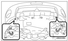
The front tie-down hooks are located between each of the front tires and the front bumper.
