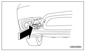
5. Screw the towing hook into the thread hole until the threads can no longer be seen.
