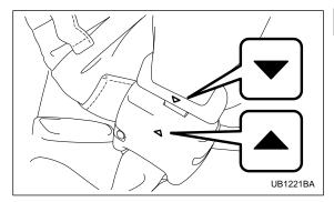
4. After fastening the seatbelt, make sure that the " $\mathbf{\nabla}$ " mark on the connector (tongue) and the " $\mathbf{\Delta}$ " mark on the buckle face outwards.
