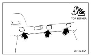
Three tether anchorages, i.e., ones for the right, center and left positions, are already installed on the rear edge of the roof.
