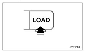
1. Briefly press the "LOAD" button. If the magazine in the player has an idle position where you can insert a disc, the disc number indicator associated with the idle position will blink.
