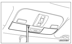
1. Remove the lens by prying the edge of the lens with a flat-head screwdriver.
