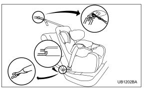
Your vehicle is equipped with four lower anchorages (bars) and three upper anchorages (tether anchorages) for accommodating such child restraint systems.
