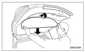
2. Hold both sides of the bottom edge of the rear gate board, rotate the rear gate board toward you, and pull it out downward.
