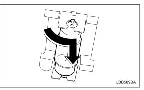
2. Turn the bulb until the flat surfaces at its ends are aligned vertically. Pull the bulb straight downward to remove it. Install a new bulb.
