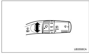
When the wiper switch is in the "  $\nabla$  " position, turn the dial to adjust the operating interval of the wiper.
