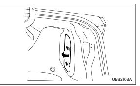
1. Push the knobs of the cover to open the cover.
