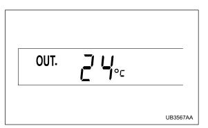
The outside temperature indicator shows the outside temperature in a range from -22 to  $122^{\circ}F$  (-30 to  $50^{\circ}C$ ).
