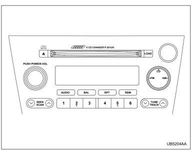
The radio will operate only when the ignition switch is in the "ACC" or "ON" position.
