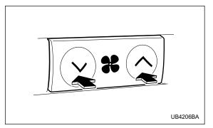
The fan speed control button has the 7 positions: AUTO position and 6 different fan speed positions. The fan speed is shown by the display.
