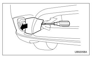
4. Likewise, insert the screwdriver still wrapped with cloth or vinyl into the cutout between the towing hook cover and the bumper. Pry out the cover.
