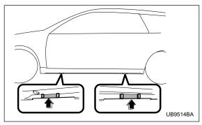
8. Place the jack under the side sill at the front or rear jack-up point closest to the flat tire.
