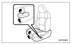
To adjust the seat cushion angle, pull up or push down the front end of the control switch. ▼ Seat height adjustment (Driver's seat only)
