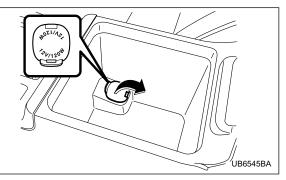
Accessory power outlets are provided in the center console and in the cargo area.
