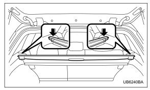
To install the cover housing, insert both ends of the cover housing into the retainers.
