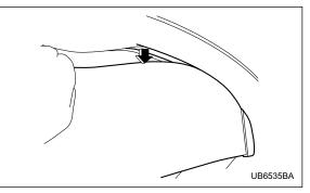
1. Remove the top of the rear gate board from the groove in the rear gate panel.
