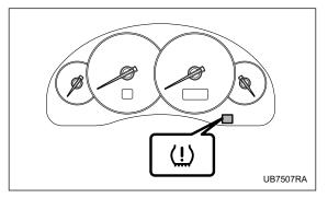
The tire pressure monitoring system provides the driver with a warning message by sending a signal from a sensor that is installed in each wheel when tire pressure is severely low.
