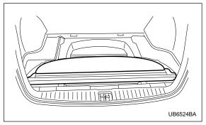
4. Stow the cover housing and rear gate board in the cargo area end.
