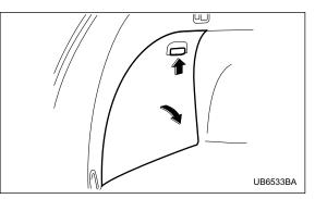
A stowage box is located on each side of the cargo area. You can access each one by pushing up and pulling the knob on the lid.
