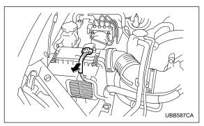
2. Unplug the connector that is attached to the top of the air cleaner case.
