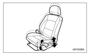
The height of the seat can be adjusted by moving the seat cushion adjustment lever up and down. When the lever is pushed down, the seat is lowered. When the lever is pulled up, the seat rises.
