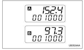
This meter display two trip meters when the ignition switch is in the "LOCK", "ACC" or "ON" position. The trip meter shows the distance that the vehicle has been driven since you last set it to zero.
