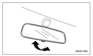
The inside mirror has a day and night position. Pull the tab at the bottom of the mirror toward you for the night position. Push it away for the day position. The night position reduces glare from headlights.
