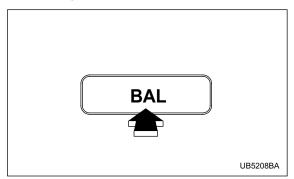
Each brief press of the "BAL" button changes control modes in the following sequence starting from volume control mode. (When the radio is first turned on, the control mode is in the volume control.)
