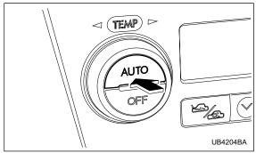
When the "AUTO" button is pressed, the indicator light "AUTO" on the display comes on. In this state, fan speed, air flow distribution, air-inlet control, and air conditioner compressor operation are automatically controlled.
